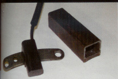
> This is the custom crank-position sensor Harrel rigged up to provide the ignition signal to the Chrysler EFI.
