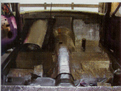
> While Harrel handled most of the drivetrain and wiring, Anna Beth laid insulation and sound-deadening over every interior panel.
